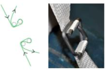
6/ Firmly hold the EMS marker and the upside part of the strip and pull down the other side until you cannot tighten the strip anymore.
